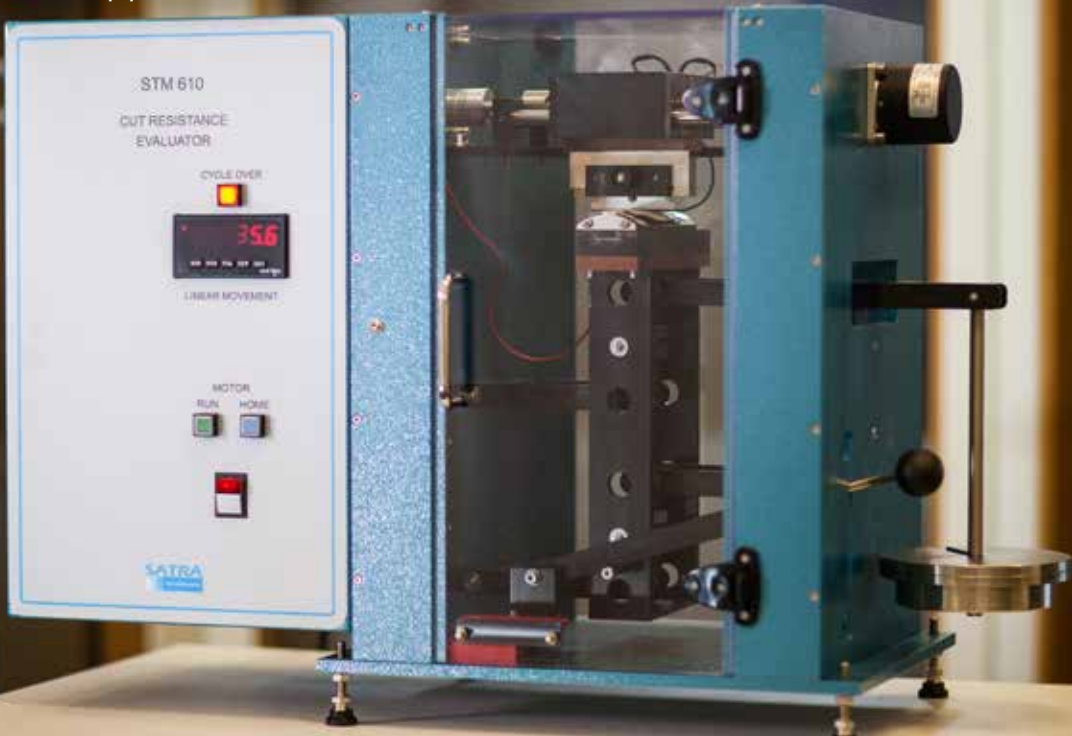
TDM test equipment
